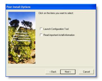
5. If you chose "Launch Configuration Tool" on the Install Options window, the installer should next launch the ATS Configuration Tool – window shown below. If you did not choose "Launch Configuration Tool" on the Install Options window, you will be able to choose this from Start > All Programs > Arbiter Time Service.
